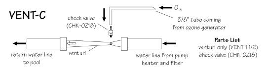
water up to and through the venturi, thereby increasing draw. On most systems, turning the valve three-quarters of the way closed should create enough suction for the unit to fuction adequately. Adjust your system accordingly (either open or close) to achieve the most desirable air draw (ideally 5 SCFH). The 1 1/2" venturi system is rated for 60 gpm with a 5 psi pressure drop.
